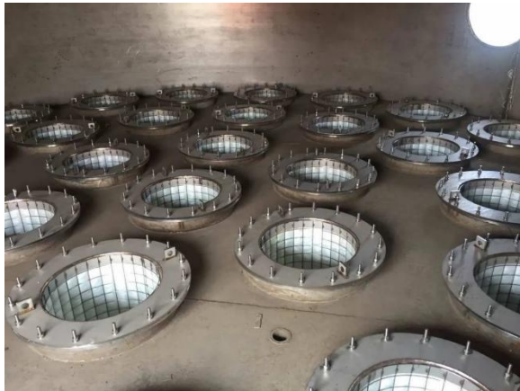
Left: finished fiber bed elements (top view) in production. Right: tube-sheet mounting layout for tower installation.
