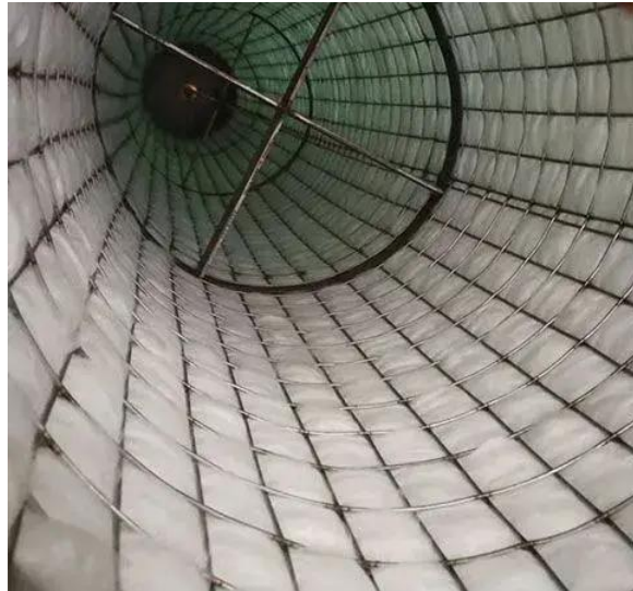
Left: assembled wire-cage fiber bed elements ready for shipment. Right: internal view of the support cage and fiber media.
