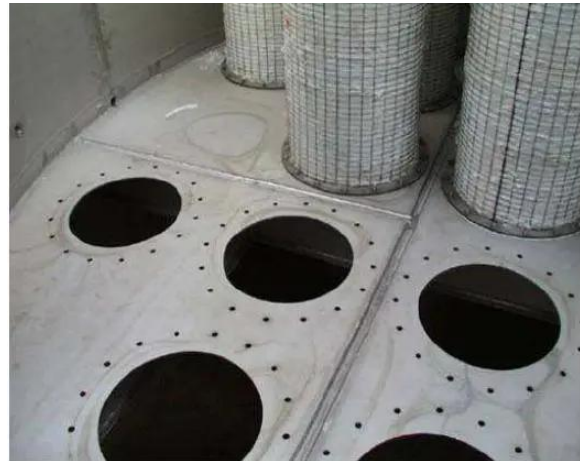
Left: finished fiber bed elements (top view) in production. Right: tube-sheet mounting layout for tower installation.
